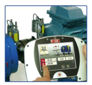
The best method of alignment is with the laser device. Due to thermal expansion and other causes such as, for example, the lubricating oil film in the plain bearings, radial thrusts by the gears etc., the position of the two shafts coupled with the machine in normal operation can be very different from their position when the machine is off and cold.
