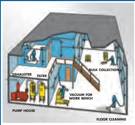
Exhauster for centralized vacuum cleaning systems
